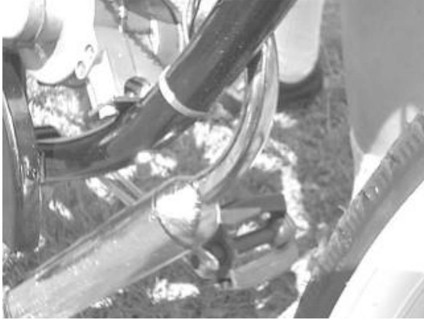
**Bike with large front frame tube:** Use 1/4" thick 1-1/8" x 2-1/2" steel plate with one hole in the center for a bolt to go through a drilled hole in tube frame and two holes for cap screws to go into engine block. Additional spacers may be required depending on the donor bike.
